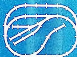
No. 26 Space—60" x 70" Track 19—Curve 14—Straight 1— \frac{1}{2} Straight 4—Left Switches 2—Right Switches
