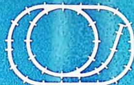
No. 28 Space—45" x 70" Track 23—Curve 5—Straight 3— \frac{1}{4} Straight 1— \frac{1}{2} Curve 2—Left Switches 1—Right Switch
