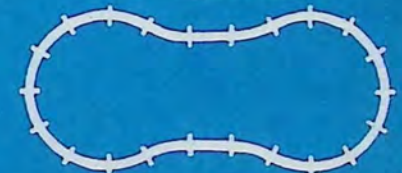
No. 25 Space—50" x 70" Track 20—Curve 9—Straight 3—Left Switches 2—Right Switches
