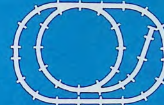
No. 28 Space—45" x 70" Track 23—Curve 5—Straight 3— \frac{1}{2} Straight 1— \frac{1}{2} Curve 2—Left Switches 1—Right Switch
