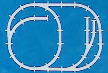
No. 25 Space—50" x 70" Track 20—Curve 9—Straight 3—Left Switches 2—Right Switches
