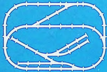
No. 22 Space—60" x 90" Track 26—Straight 38—Curve 4— \frac{1}{2} Straight 5—Left Switches 3—Right Switches
