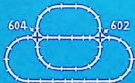
No. 1—Space 67-1/2" x 105" Track 24 Curve 11 Straight 2-1/2 Straight 1 Crossover Train Control Crossover This layout allows the operation of two trains at the same time. A Train Control Crossover is used to prevent collisions.
