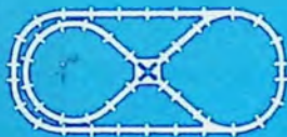
No. 5—Space 46" x 100" Track 21 Curve 14 Straight 4-1/2 Straight 2-1/2 Curve 1 Crossover and 1 pair of Switches
