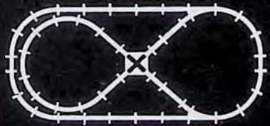
No. 5—Space 46" x 100" Track 21 Curve 14 Straight 4½ Straight 2½ Curve 1 Crossover and 1 pair of Switches
