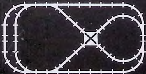
No. 20 — Space 65" x 130" Track 22 Curve 4 - ½ Curve 26 Straight 5 - ½ Straight 3 pair of Switches 1 Crossover
