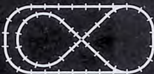
No. 3 90" x 42" 21 Curve Track 2-1/2 Curve Track 20 Straight Track 2-1/2 Straight Track 1 Crossover 1 pr. Switches
