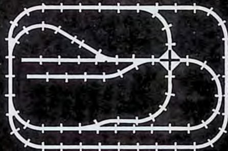
No. 10 Space 80" x 120" Track Required 30 Curve 42 Straight 1-½ Straight 3 pr. of Switches 1 Crossover
