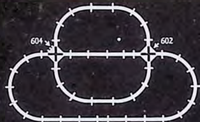
No. 1—Space 67½" x 105" Track 24 Curve 11 Straight 2-½ Straight 1 Crossover 1 Train Control Crossover
