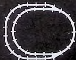
No. 3 60" x 140" 32 Curve Track 27 Straight Track 1 pair Switches 1 Crossover
