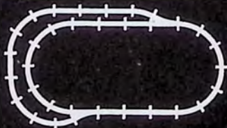
No. 12—Space 50" x 90" Track 20 Curve 10 Straight and 1 pr. of Switches
