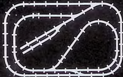
No. 18 — Space 70" x 110" Track 28 Curve 39 Straight 4-1/2 Straight 3 pair of Switches
