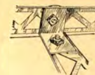
Fig. 6. Right Angle Connection for Branch Girders.
