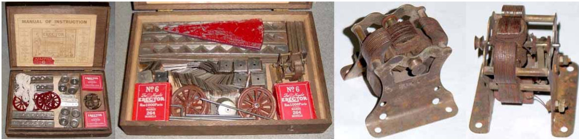
1914 #6 set. Inside top layer and manual on the left, bottom layer in the middle. Note the large propeller blades. This was the only year the P51 motor was available (two pictures on the right). Note the single “foot” or flange across the bottom of the base and the brass strip brushes.
