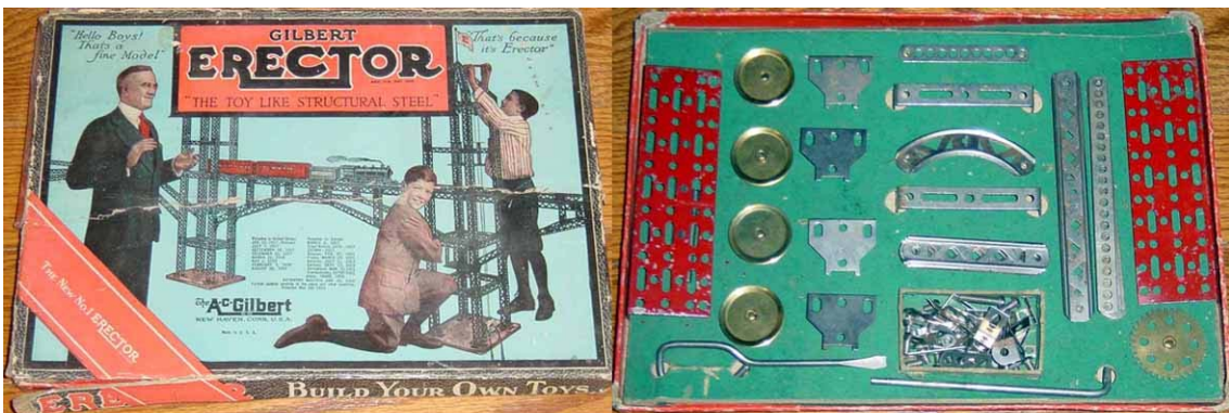
1927 #1 set. The gear teeth got finer this year. For example, the CJ 24 tooth gear became a 36 tooth gear. The other gears and P52 ladder chain had similar changes.
