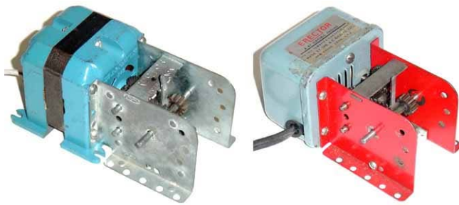
The A49 motor on the far left was included in sets #6 1/2 and larger from 1938 - 1964. The exception was when the A47 shown on the near left was substituted from 1950 - 1953. Both motors went through changes during their runs in case color, gear box side plate color and gear box design.
