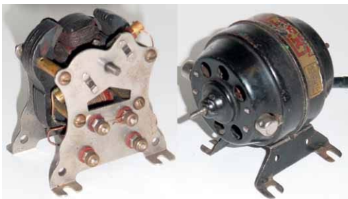
The P58 AC/DC motor on the far left and the P56G 110V motor on the near left were staples for powering models for years. The P58 was introduced in 1915, the P56G in 1923. Both continued to be used in sets into the early 1940's.
