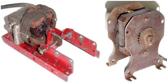
The P51 Electric Engine on the far left and A52 induction motor on the near left powered the models in 1935 - 1937. The P51 showed up in Sears sets from 1938 - 42 also. The open armature of the P51 makes it a favorite of collectors.
